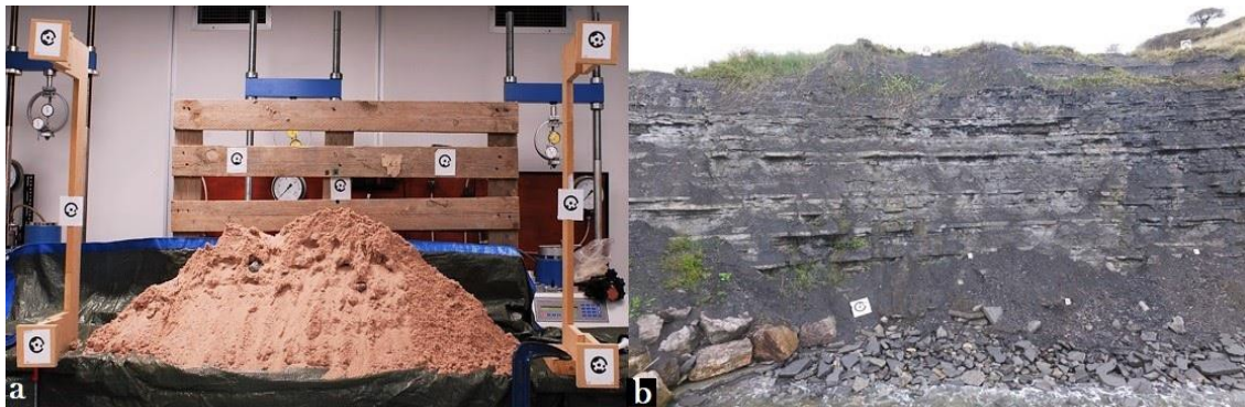
Figure 1: a) Lab experimentation: the slope was composed of sharp sand and was 1.5m long, 0.5m wide, 0.5m high and with a gradient of 60°. b) A section (25x20m) of an unstable sea cliff was selected for field verification.
