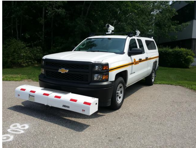
Figure 2: ARAN 7000 Vehicle owned and operated by the MTO. The end goal of research is to attach a camera rig to a mobile vehicle allowing automated network level data acquisition for rockfall prone highway corridors.
